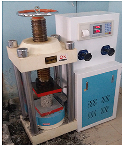
Figure 4: Compressive strength test setup
